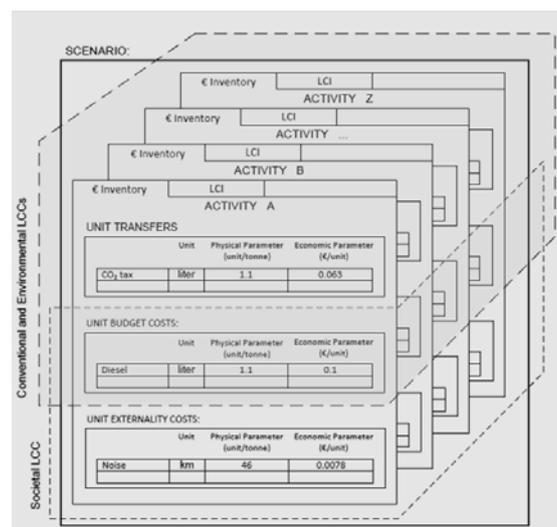
**Figure 1:** Overview of the cost model structure, illustrating a range of activities (A through Z) and the cost coverage of Conventional, Environmental and Societal LCCs from Martinez-Sanchez et al. (2015).<sup>i</sup>
