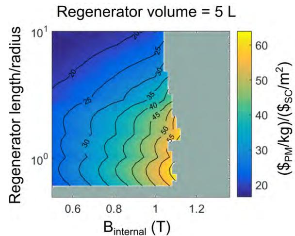
Figure 2: The factor between the price of the superconductor tape per m<sup>2</sup> and the price of the permanent magnet per kg.
