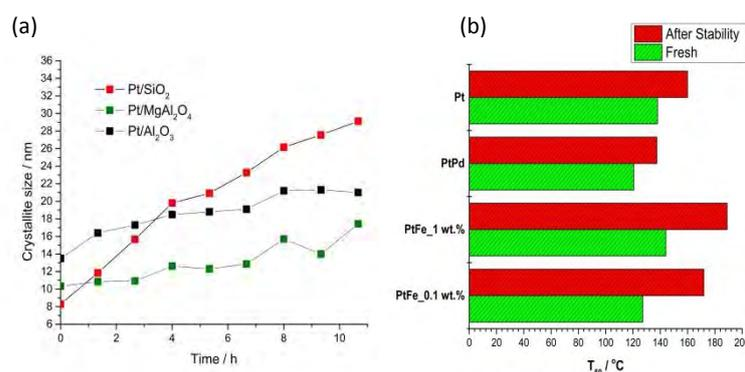
Figure 1 – (a) Crystallite size of Pt on different supports from *in situ* XRD measurements; (b) Temperature of half conversion (T<sub>50</sub>) for Pt/SiO<sub>2</sub> and PtX/SiO<sub>2</sub> (X=Fe and Pd).
