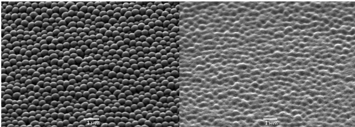
*Figure 1: A nanostructured nickel tool insert (left) and a polypropylene replication (right) made by injection moulding without applying induction heating to the tool. It is obvious that replication is not as sharp as the tool, but this can be dramatically improved by introduction local heating of the tool insert.*
