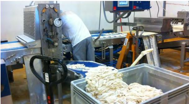
Figure: 1: Waste material due to height differences on the belt (fixed with the fellow fork truck)
