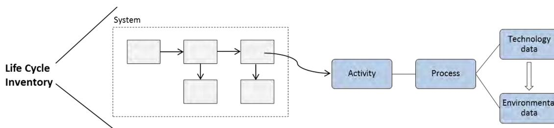
**Figure 1** Structure of LCI data. Boxes within the studied system represent processes in the life cycle of a technology. Blue boxes show the data layers: Activity) Societal need to be fulfilled; Process) Industrial step in the system; Technology data) Exchanges of economic goods between processes, Environmental data) Environmental exchanges caused by the economic exchanges.
