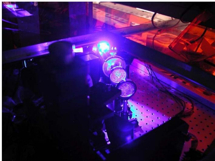
Figure 1. The recently developed 3D polychromatic stereolithography printer at DTU Nanotech can expose with multiple wavelengths, here 365 nm and 450 nm, at  $<15\ \mu\text{m}$  pixel size to freely combine multiple materials within a printed object.
