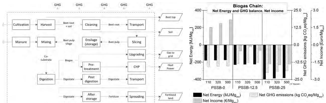
Figure 1 – Biogas production chain (left) and results for integrated energy, GHG, and economic analysis (right), taken from Boldrin et al. (2015).
