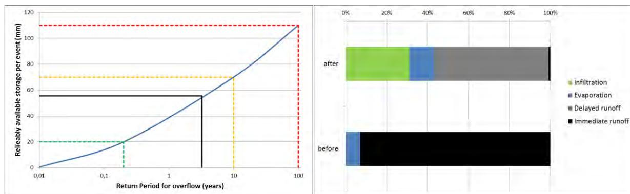
Figure 1: Example outputs. To the left: Key indicator 1 – volume of runoff/return period at the single event scale. To the right: Key indicator 2 - annual water budget before and after.
