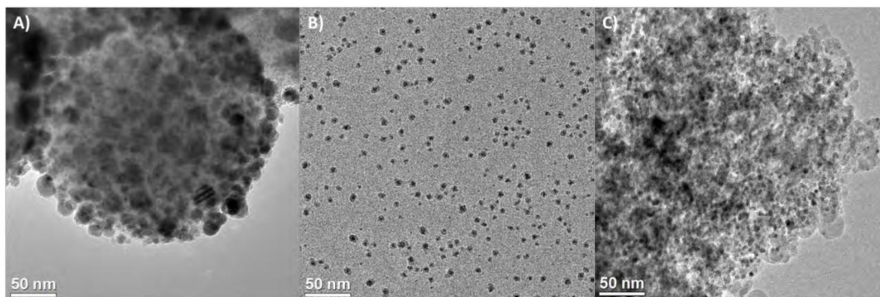
TEM micrographs of NiGa NPs supported on A) 200 nm SiO<sub>2</sub> spheres, B) SiO<sub>2</sub> membranes and C) High surface area SiO<sub>2</sub> support.
