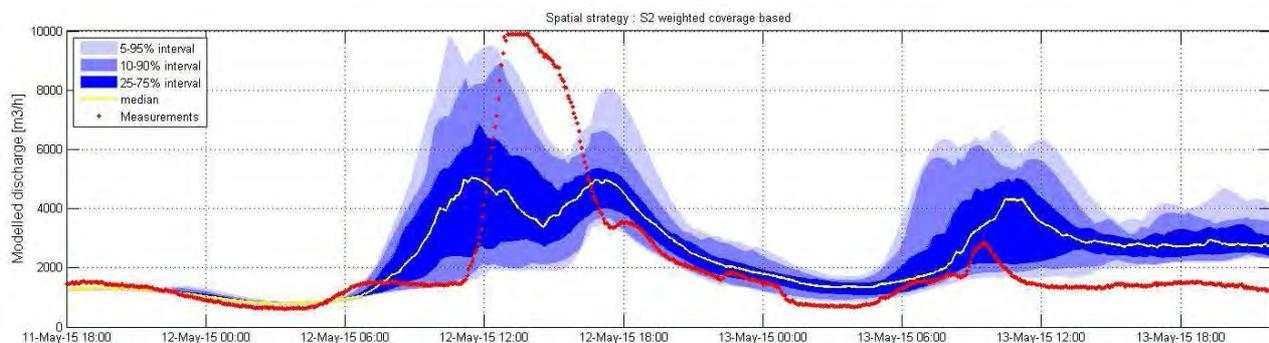
Figure 1: Flow prediction at Damhuså catchment generated the 11<sup>th</sup> of May 2015 at 18:00 using the DMI-HIRLAM-S05 NWP model
