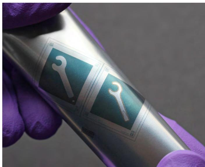
Flexible plastic foil with embedded plasmonic color meta-surface decoration. The color appears from a thin film of aluminium deposited on top of a nanotextured surface.
