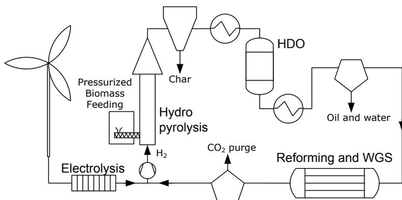
**Figure 1** Proposed process diagram including catalytic hydrolypyrolysis, char separation, temperature adjustment, deep HDO, liquid separation, pyrolysis gas reforming and water gas shift (WGS). Additional hydrogen may be obtained from water electrolysis.
