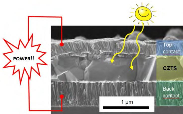
Figure 1. Cross-sectional view of a CZTS solar cell produced by our group.
