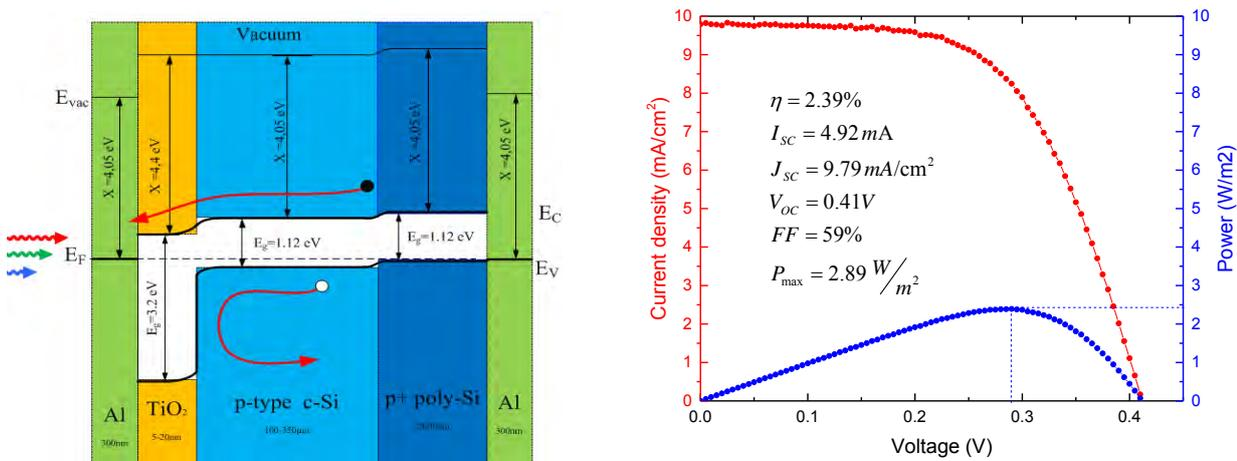
**Figure 1:** Energy band diagram of TiO<sub>2</sub>-Si-poly Si structure (left), current-voltage and power –voltage characteristics (right)
