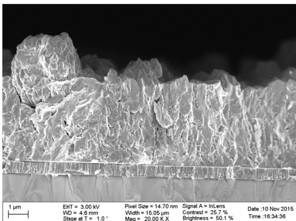
Fig. 1: SEM cross-sectional image of a CZTS layer identical to the one used in a 0.2 % efficient solar cell. The CZTS layer (4-5  $\mu\text{m}$  thick) is deposited on a 500 nm layer of Mo that has been sputtered on soda lime glass.
